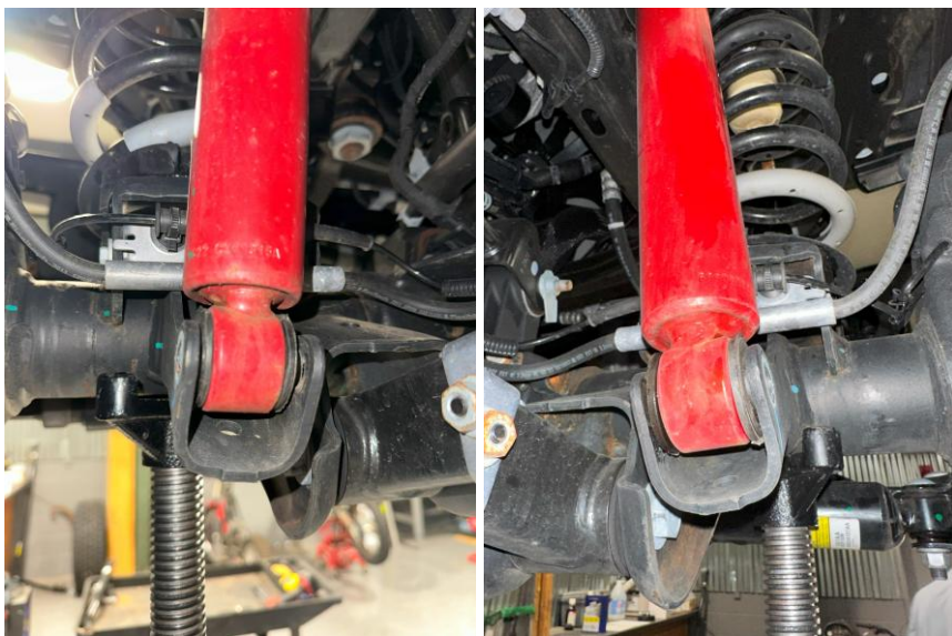
Figure 4: Front driver/passenger lower shock bolts removed
