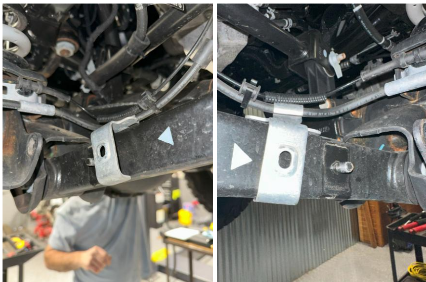
Figure 6: Front driver/passenger lower brake line mount removed
