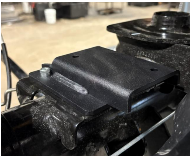
Figure 31: Bump-stops (1" tall and 3" tall bump-stop options)
