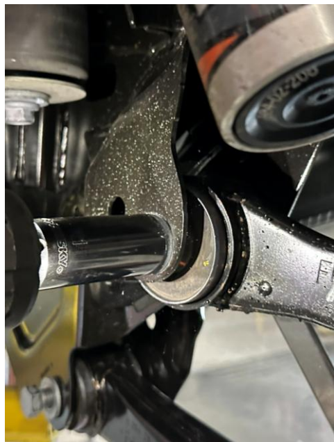
Figure 24: Rear control arm bolt locations (2 arms each side, 4 bolts per side, or 8 bolts total)
