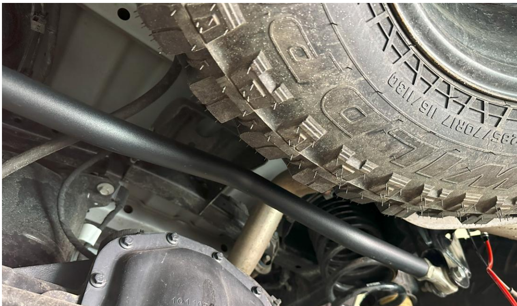
Figure 30: New rear track bar installed
