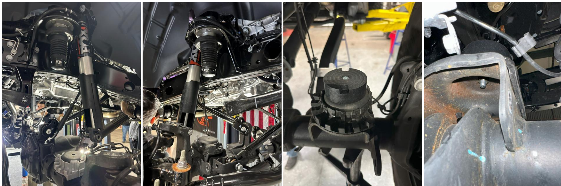
Figure 10: Axle drooped with old springs removed, and bump stops installed
