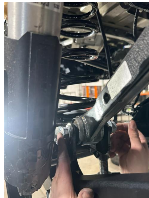
Figure 24: Rear control arm bolt locations (2 arms each side, 4 bolts per side, or 8 bolts total)
