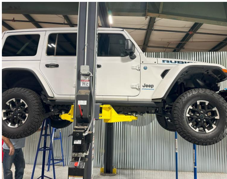
Figure 18: Vehicle rear axle supported by lift and jack stands
