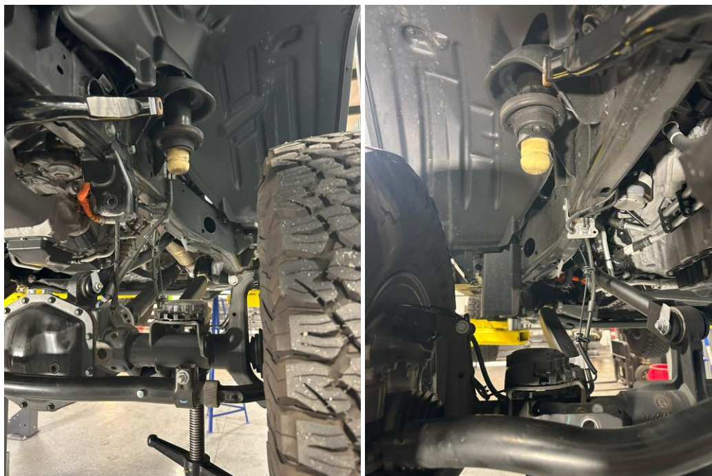
Figure 9: Axle drooped with old springs removed
