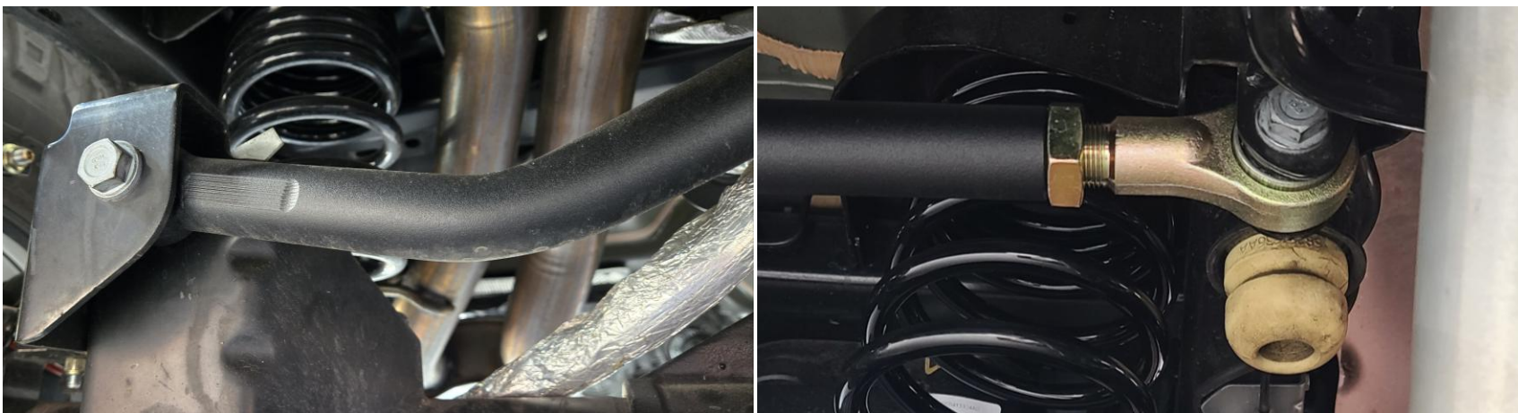
Figure 29: New rear track bar installed
