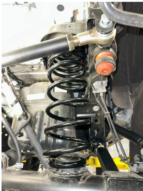
Figure 25: Axle drooped with old springs removed, and bump stops installed
