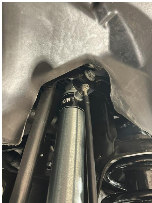
Figure 11: Front shock top and bottom bolt installed loosely
