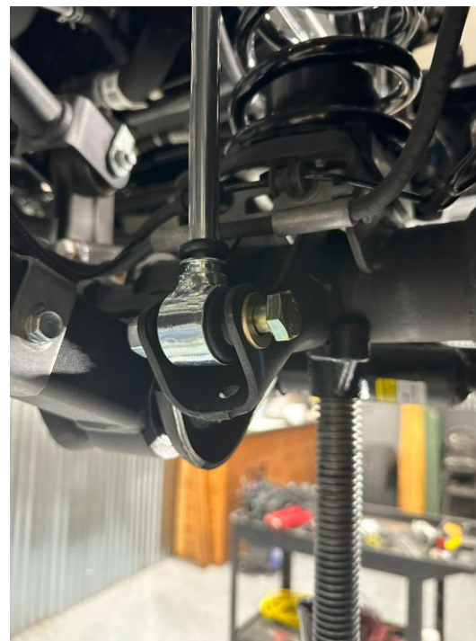
Figure 11: Front shock top and bottom bolt installed loosely
