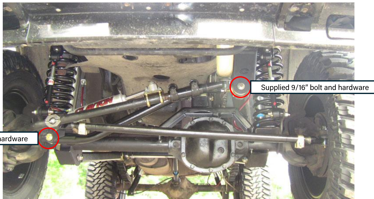
XJ drop bracket and track bar fully installed and painted
