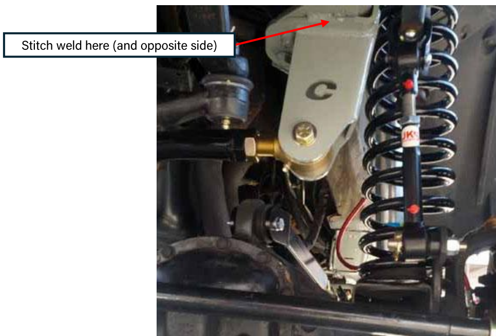
XJ frame-side drop bracket weld locations
