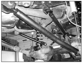
21. Remove the upper control arms from the front axle and frame. Retain the nut tab from the frame mount.
