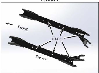
9. With the subframes properly mounted in position, using the holes in the subframes as a guide, mark the horizontal mounting holes (Fig 6) to be drilled in the frame (4 holes total).
