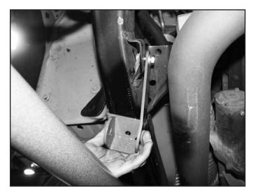
23. Drill 3/8" holes at the two marks on the outside surface of the frame. Drill the holes all the way through the frame.
