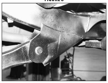
19. Locate (2) pre assembled long lower control arms (A220). Adjust the length to 29-1/4". Install a provided 90° grease zerk (60107) in the flex end so it faces 45° from facing down the arm and towards the outside of the vehicle. The arms are installed with the flex eye at the frame with the bend towards the inside of the vehicle.
