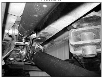
12. Locate the OE mounting tabs on the two emergency cables (Fig 13). Using a cut-off wheel, etch the side of the bracket so that it can be easily formed open and removed from the cable. Leaving the cable free at these points will eliminate the chance of binding during extreme suspension articulation. Take care not to cut into the cable.
