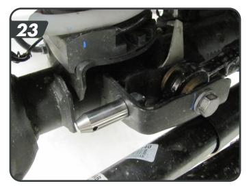
o. Install the longer disconnect post on the driver side axle sway bar link mount with it pointing inboard [24]. Fasten with the  $\frac{1}{2}$ " nylock nut and tighten to 64 ft-lbs. Tighten the post with the pin hole parallel to the ground. Slide the polyurethane spacer on the pin up against the axle tab.
