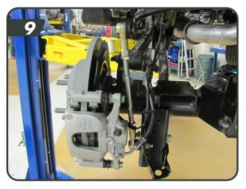
c. Install the rear bump stop spacers on the axle. Fasten the bump stop spacer to the axle with the 5/16" x 1-1/4" bolts, nuts and washers. Torque bolts to 15 ft-lbs. (1/2") [10]
