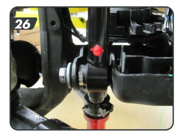
w. Install the remaning longer sleeve on the driver side and slide the polyurethane spacer onto the sleeve so it will mount towards the axle mount tab. Install the quicker disconnect to the inboard side of the axle tab with the original sway bar link hardware.
