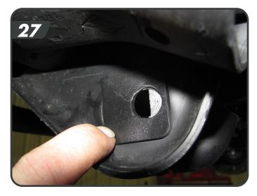
ab. Re-install the control arm to the axle with the factory bolt with cam lock washers. Rotate the cam lock so that the bolt will be as far back in the slot as possible (most rearward setting = max caster). [28] Snug the cam hardware so that the cams are retained within the stops. Final torque will be completed with the weight of the vehicle on the suspension.
