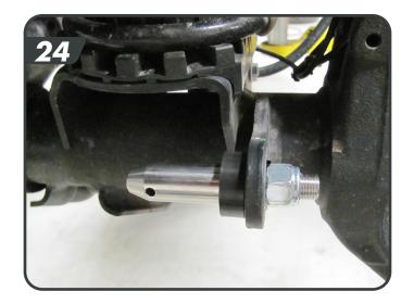
p. The kit comes with disconnect retention brackets to hold the links when the links are disconnected. Install the retention brackets using the provided 5/16" bolts into the factory hole in the front of the coil bucket [25]. These are designed to slightly interfere with the edge of the coil bucket to hold them in place.
