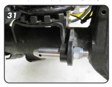
The kit comes with disconnect retention brackets to hold the links when the links are disconnected. Install the retention brackets using the provided 5/16" bolts into the factory hole in the front of the coil bucket [32]. These are designed to slightly interfere with the edge of the coil bucket to hold them in place.
