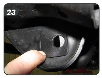
d. Re-install the control arm to the axle with the factory bolt with cam lock washers. Rotate the cam lock so that the bolt will be as far back in the slot as possible (most rearward setting = max caster). Snug the cam hardware so that the cams are retained within the stops. Final torque will be completed with the weight of the vehicle on the suspension. [24]
