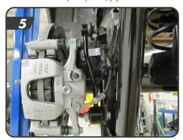
i. Remove the rear inner fender liners by removing the 3 bolts (8mm) to gain access to the upper shock bolt [6]. **Note: Some models may require the parking brake cables be disconnected at the wheel to gain adequate slack.**
