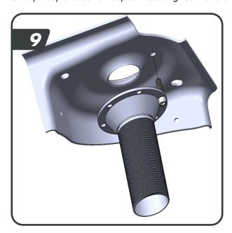
f. Using the Cone Adapter Plate as a template, accuratly mark the 5 remaining hole locations on the upper spring mount.
