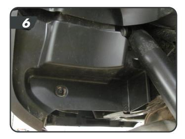
Support the axle with a jack under the center of the differential and remove the shocks from the frame and axle (18mm), save hardware [7].
