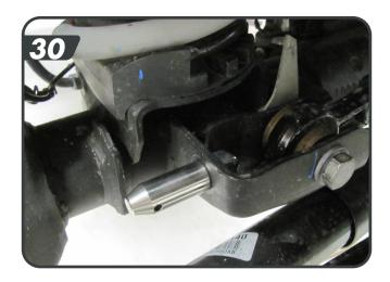
Install the longer disconnect post on the driver side axle sway bar link mount with it pointing inboard [31]. Fasten with the ½" nylock nut and tighten to 64 ft-lbs. Tighten the post with the pin hole parallel to the ground. Slide the polyurethane spacer on the pin up against the axle tab.
