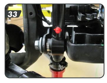
ac. Install the remaning longer sleeve on the driver side and slide the polyurethane spacer onto the sleeve so it will mount towards the axle mount tab. Install the quicker disconnect to the inboard side of the axle tab with the original sway bar link hardware.
