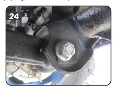
Repeat cam bolt installation on the driver's side.
