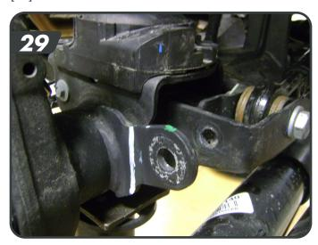
t. Install the shorter passenger side post on the side of the track bar mount at the sway bar link mount location with it pointing outboard [30]. Fasten with the ½" nylock nut and tighten to 64 ft-lbs.
