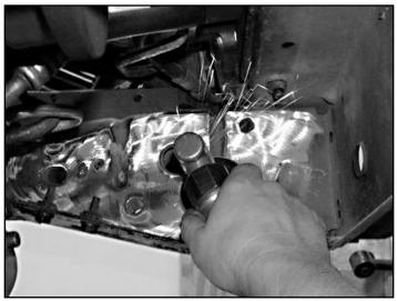
Z Test fit the Inner and Outer Chassis Plates (A & B) again to check for flush fitment against chassis surface, and to ensure all debris has been removed from the necessary areas.
