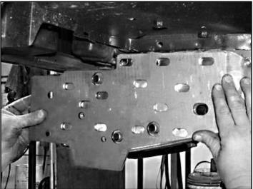
Z Place the supplied Installation Spacers (F) on the Steering Gear Mounting Bolts (D) and temporarily insert bolts into Support Sleeves (C) from the outboard side of chassis. *HINT:* Recessed side of Installation Spacer (F) should face Outer Chassis Plate (A).
