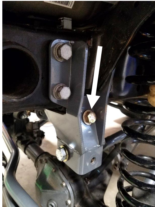
Figure 8. Installing Upper Track Bar Mount Hardware
