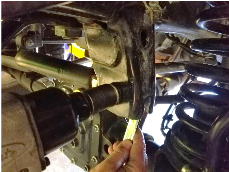
Figure 1. Removing Frame Side Track Bar Bolt
