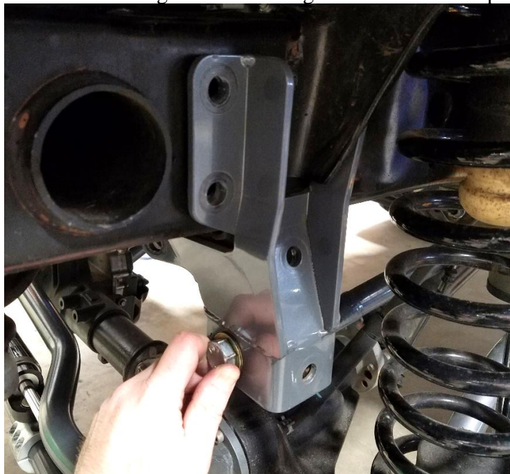
Figure 6. Synergy Track Bar Brace Loosely Installed
