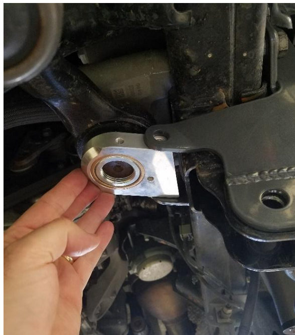
Figure 12. Installing Synergy Sector Shaft Brace on Pitman Arm Nut
