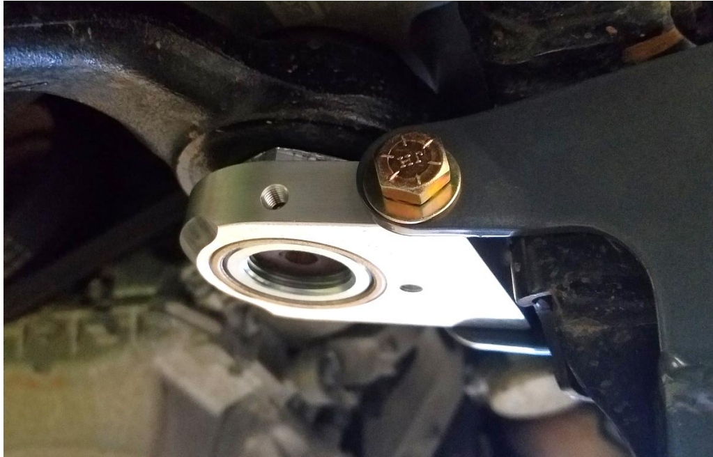
Figure 13. Installing Hardware in Synergy Sector Shaft Brace
