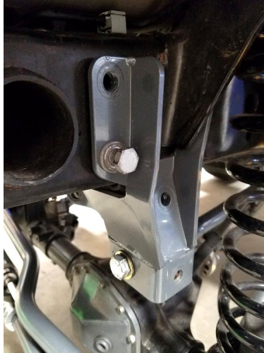
Figure 7. Threading Bolts into Steering Box
