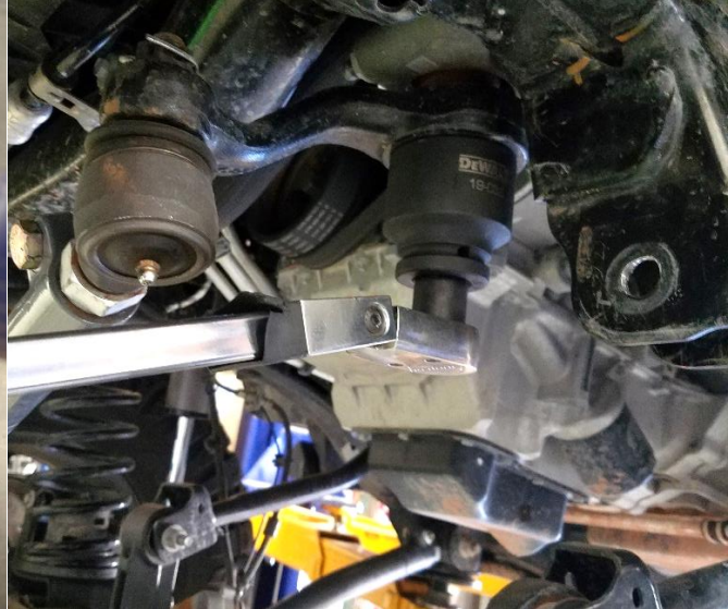
Figure 5. Torquing Pitman Arm Nut
