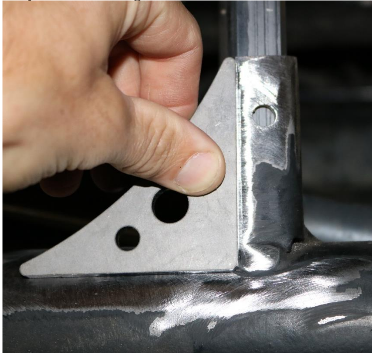
Figure 4. Paint Removed from Areas to be Welded (From Rear of Vehicle)
